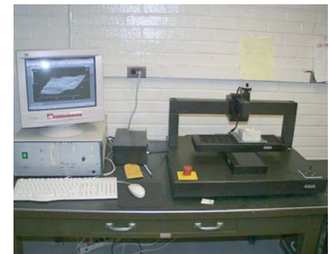
Laser profilometer with a data acquisition system
